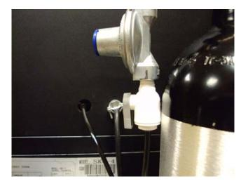
5. The maximum length of the tube can be 50 ft. You may need to adjust the gas pressure accordingly: remove the cap, and turn the adjustment clockwise to increase the pressure until the wine flow is sufficient.
