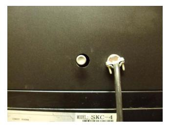
3. Use ¼" OD tube to connect the gas inlet at the unit and the gas outlet at the pressure regulator valve.
