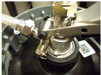
2. Turn the keg coupler clockwise until 2 mounting tabs lock over the slide—up ramps.
