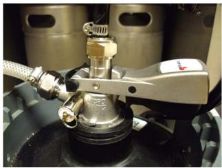
4. Open the pressure regulator valve by turning it counter-clockwise.
