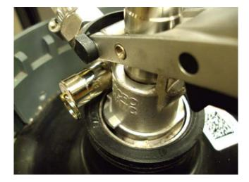
3. Press down the coupler lever handle to turn on the gas and wine ports.
