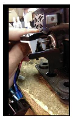
5. Install new overload. On the backside center, there is a circular receptable for peg to slide into.
