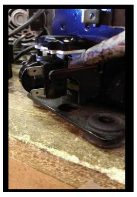
3. First remove the relay, gently wedge flathead between back of relay and compressor.
