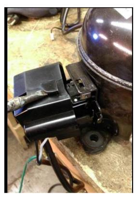
1. With flat head screw driver, insert the tip underneath black lip and push into it. Once you have the leverage, pull it up. It should unhook.
