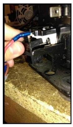
6. Install new relay in same manner. There are two holes on backside of relay, and the two lower pegs would slide into the back of relay.
