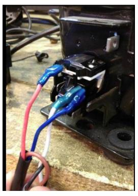
2. The top piece is the overload (half white/black). The bottom piece is the relay starter (all black piece). Please take note of the colored wires: red wire to overload, white/blue combo wire to relay.
