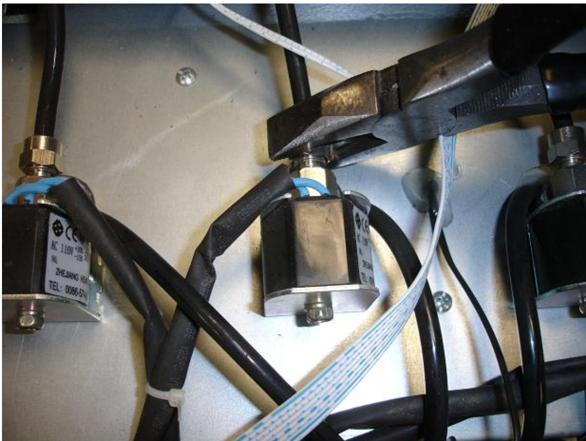
Loosen the tube nut.
