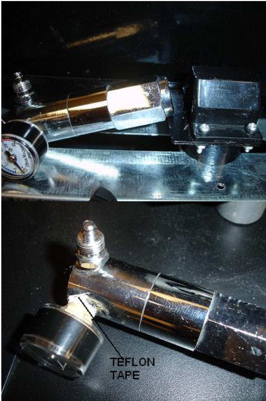
Remove the gauge and then install it on the new regulator with Teflon.
