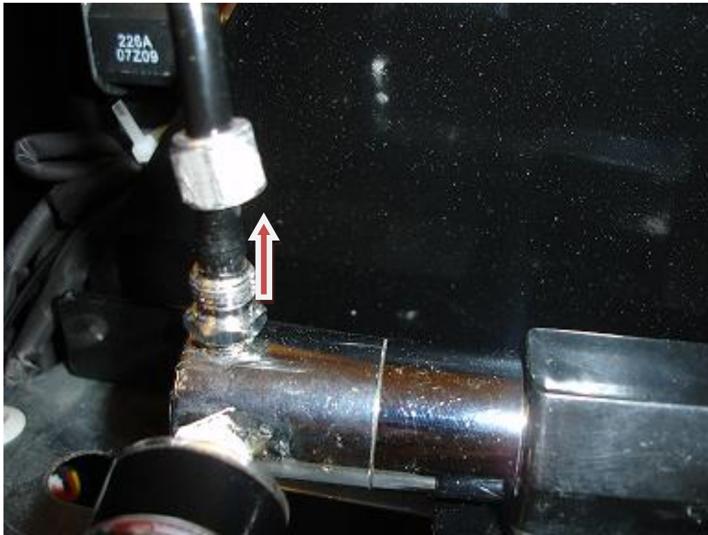
Loosen the nut tube at the top.
