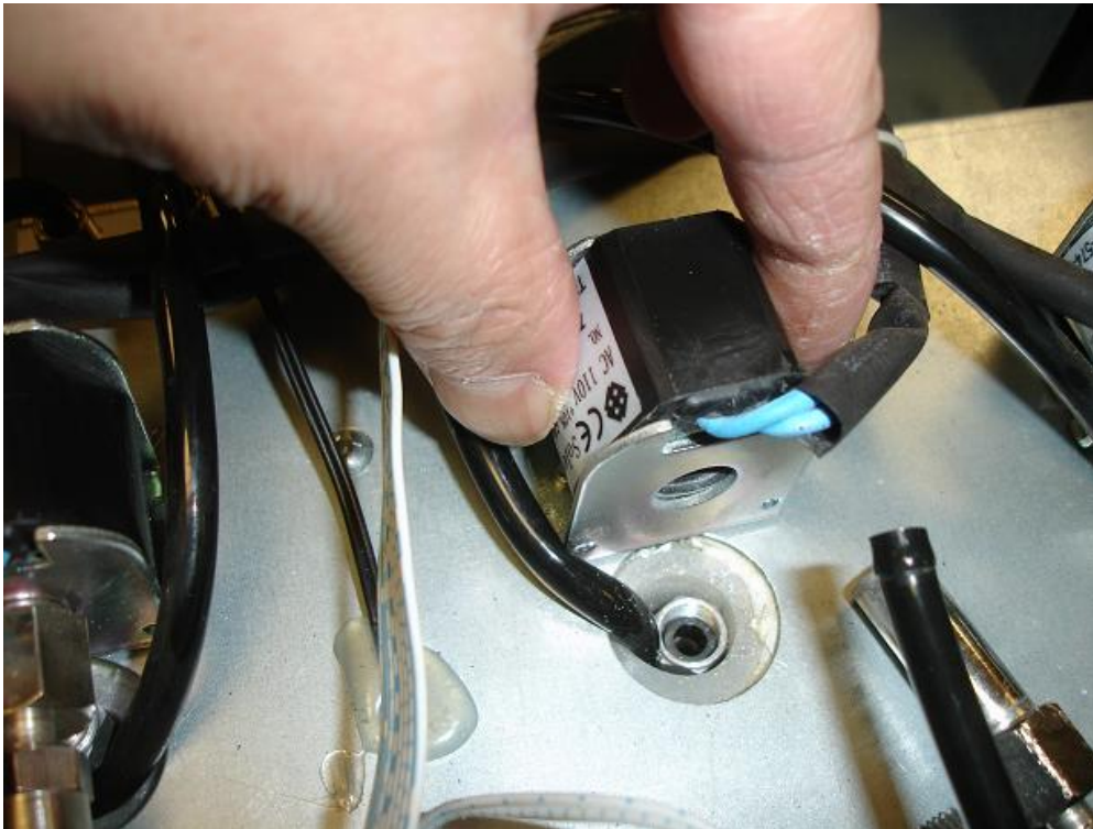
Pull and remove the coil.
