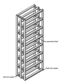
Step 2: (Attaching remaining shelves to end ladders) Place the other seven shelves onto the remaining seven rungs and attach in the same way as in Step 1. Make sure the shelves have the trim pieces are facing the front.
