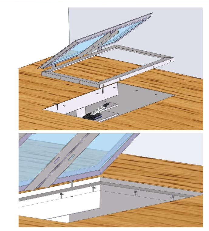
The electric motor is installed with the bolt, which is located in the frame's slots, and mounted, so that the fully extended motor arm places the lid in an 85 degree angle (see above figure).
