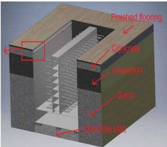
In the case of underfloor heating, the heating tubes must not be closer than 400mm to the wine cellar as the heat from these will interfere with the delicate climate of the wine cellar.
