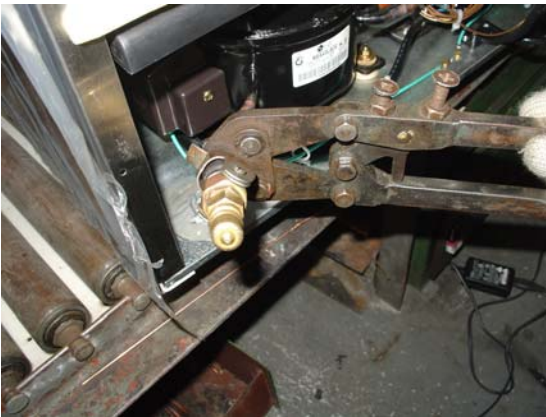
1-4-23. Clamp the process tube and make it flat, and seal it after ensuring no leakage of the gas.
