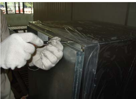
1-4-24. Connect the refrigeration system to power and check whether there is any problem and then fix the back panel
