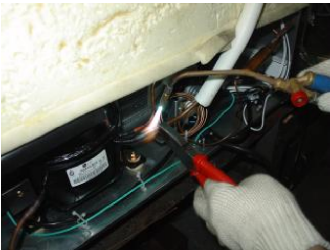
i. Test with towel as charging Ni trogen until there are no bubbles.
