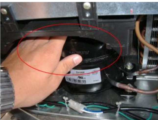
(5) If exhaust pipe isn't hot felt by hand after compressor running a period of time.
