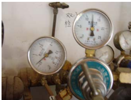
1-4-7-6、 Charge nitrogen. Connect the dried Nitrogen with the pressure is 1Mpa to the process tube
