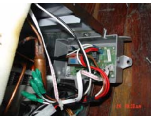
6-1-5、 Take off the upper cover of the control board.
