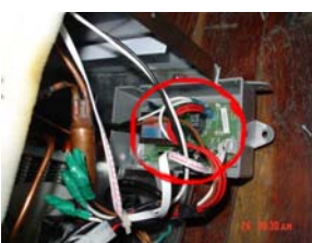
6-1-6、 Pull out the terminal on the control board.
