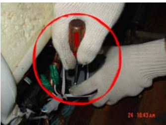
6-1-4、 Take off the screws of the control board.
