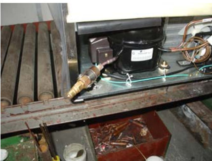
1-4-7-6、 Charge nitrogen. Connect the dried Nitrogen with the pressure is 1Mpa to the process tube
