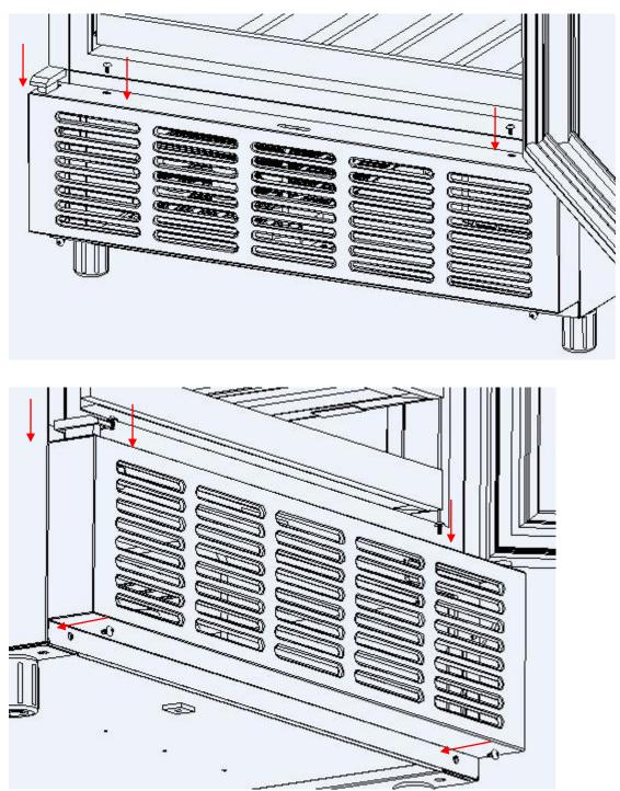
6. Take out the screws from the accessory bag and add the grill to the cooler using the screws provided (see detailed positions as shown in the image above). Add the plastic door support on the grill as shown.
