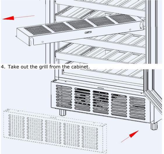
5. Assemble the grill in the right position as shown in the image above.
