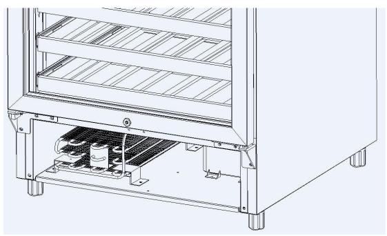
1. Check the lock. Make sure the spring bolt is inside the glass door frame. If it is outside, use the key to turn it into the glass door frame.
