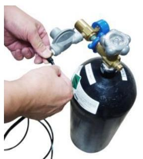
STEP 9: Insert the gas hose to the connect of the regulator.
