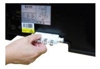
STEP 5: Firmly press the manifold to the back of the open cooler and ensure that it is fastened securely.
