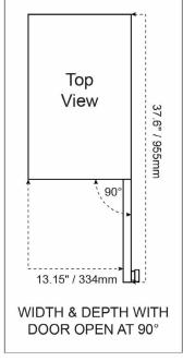
\*Please note: the unit depth with handle, when door is closed, is 24-7/8" (632 mm)
