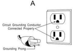
It is not recommended to use this beverage cooler with an extension cord or power board. Please ensure that the appliance is plugged directly into the electrical outlet.
