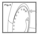
When the temperature of the aluminum container has reached the set temperature, the blue and red LED lights on the control panel will both turn off – leaving only the green LED light that indicates the set temperature will be on.
