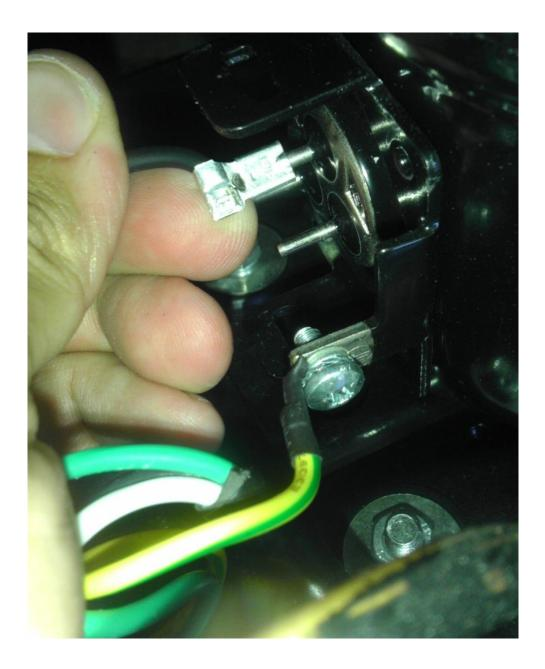
\*\*\*\*PLEASE NOTE: THE OVERLOAD WILL HAVE A 3 INCH BLACK WIRE WITH A FEMALE CONNECTOR THAT WILL CONNECT DIRECTLY TO THE TOP UPPER PIN.
