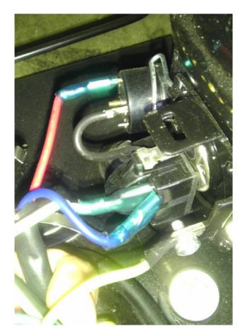
With a flat-head screwdriver, wedge the components off the pegs on the side of the compressor (big black motor). Set the old components aside.
