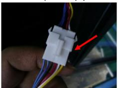
Place the wire and connection back into its housing. Please be careful not to crimp the wire.
