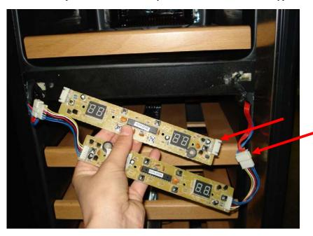
Disconnect the wiring connections.
