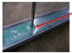
Connect the temperature display wire from two sides
