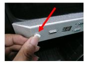
A new temperature display board is now installed
