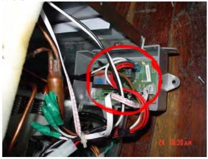
9. Place the control board cover back into position and fasten it with the screws.
