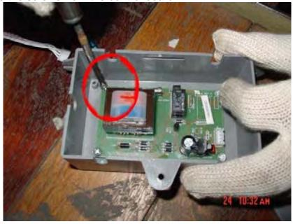
7. Replace the control board with a new one and fasten the screws.
