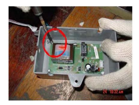
8. Connect the terminal on the control board.
