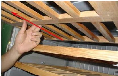
2. Remove the four screws on the evaporating board.
