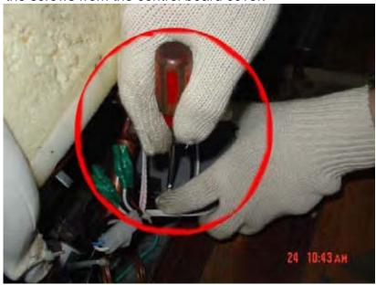
4. Remove the cover of the control board.
