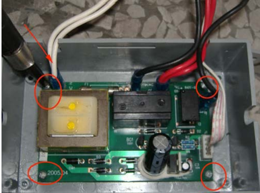
10. Plug in the terminal on the control board.
