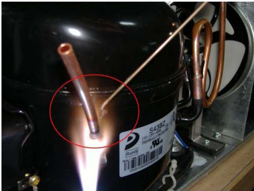
e. Connect the charging tube to the process tube.
