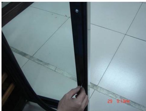
Step 4 Insert the other screw
