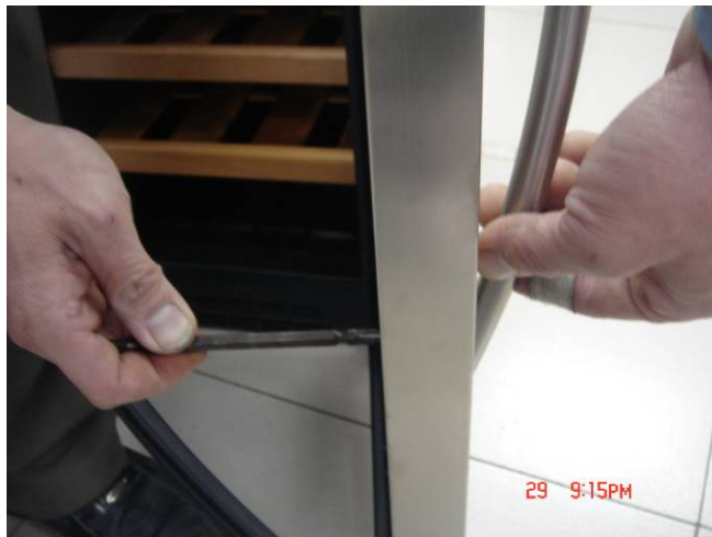
Step 6 Install the handle with second screw
