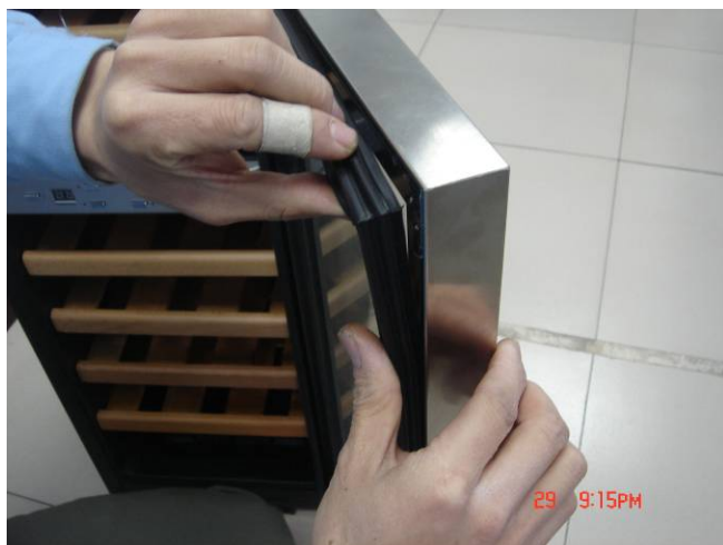
Step 7 Put back the seal
