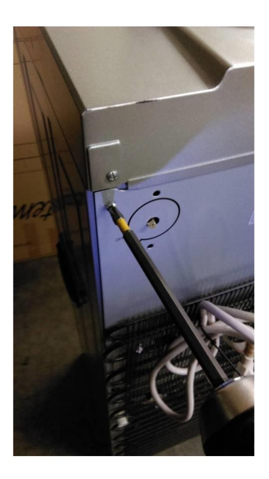
1) We would need to remove top back silver panel. There are a total of six screws, remove the four corner screws first, then the two screws that hold thermostat in place.
