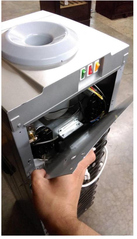
3) Next step would be to loosen up mounting screws for the condenser coil.
