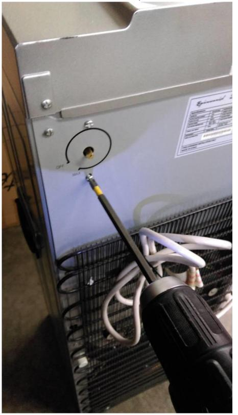
2) Once all screws are loosened up, proceed to slide the panel out of place.
