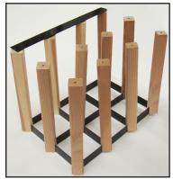
**Step 5:** Place vertical strips on dowels.
