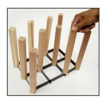
**Step 4:** Insert dowels at the other end of the rack and insert rest of horizontal strips by bisecting the rack. Insert dowels through center of rack (this keeps strips from coming out of the notches.) Install remaining dowels, working from center of the rack towards the outside.
