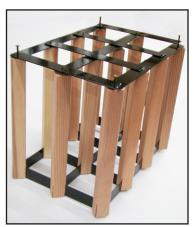
**Step 7:** Place nails in all four corners; tap lightly with hammer. (Do not drive nails around perimeter of rack.) This holds strips in place and holes aligned.
