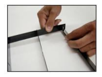
**Step 2:** Insert horizontal strips into vertical strips.
