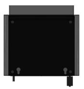
5. If you install more Modular units next to each other, connect those together by applying connection screws on the right side of the Modular. Place the next Modular on the right by sliding the slotted holes over the connection screws.
