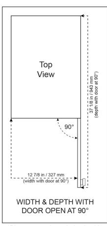
\*Please note: the unit depth with handle, when door is closed, is 24 7/8 in (632 mm)
